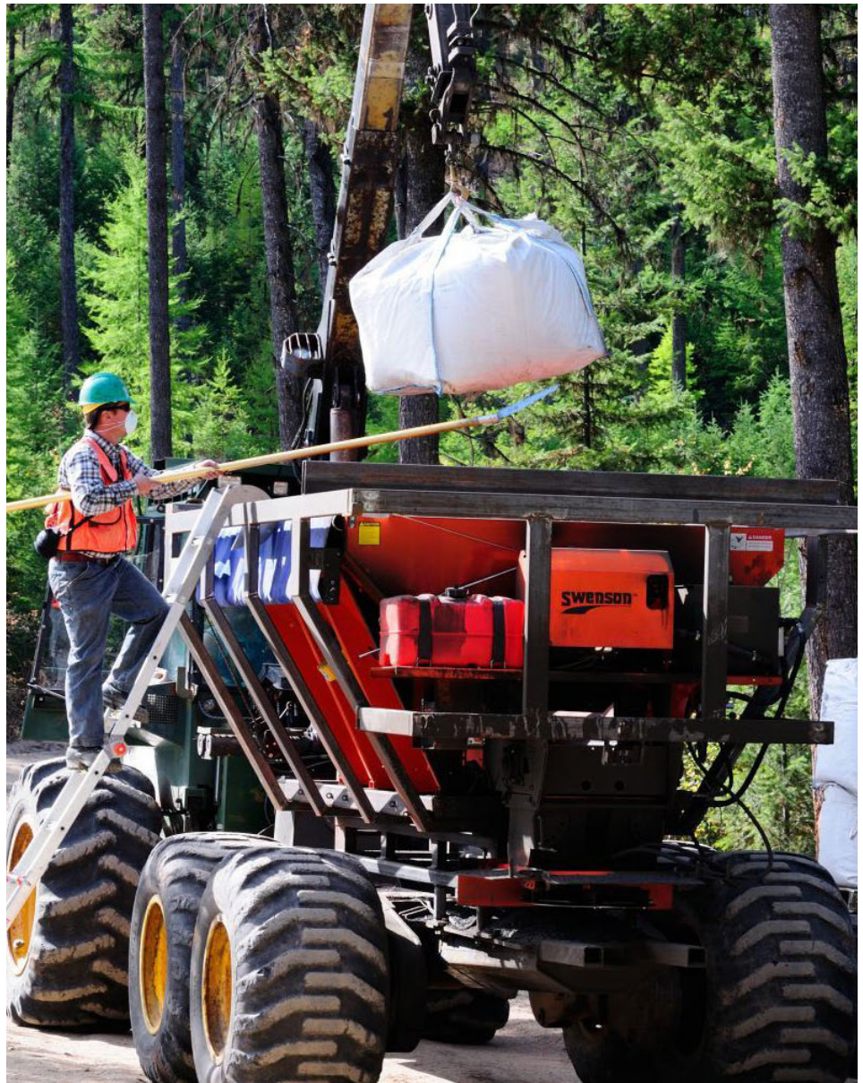
A high-capacity biochar spreader that can be mounted on a log forwarder and used on skid trails and log landings to distribute biochar has been developed by RMRS scientists and the Missoula Technology and Development Center. USDA Forest Service photo.
