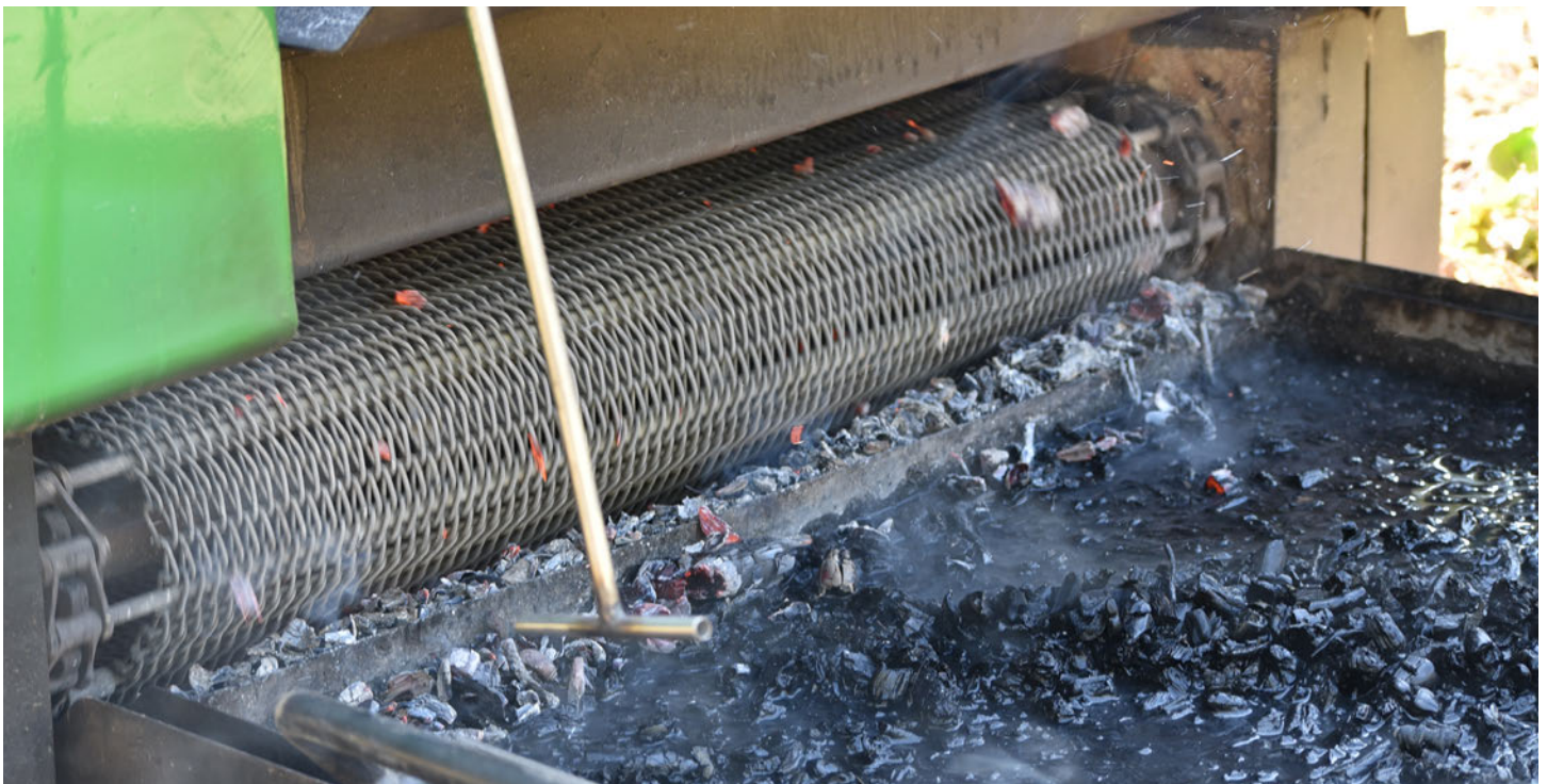
For land managers seeking solutions for implementing grassland restoration projects and hazardous fuels reduction projects, biochar is a promising product that can be the cornerstone of an organic matter redistribution system. In this photo, biochar is produced by the CharBoss, a mobile biochar processing air curtain burner. USDA photo by Darcy Weseman.
